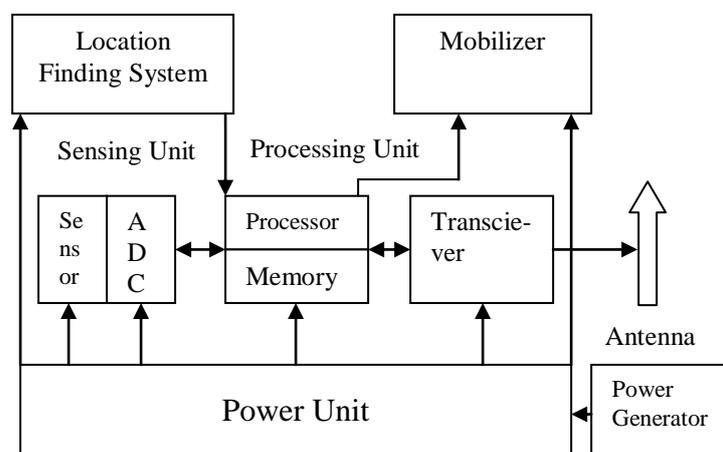
Fig 2: Block diagram sensor networks
