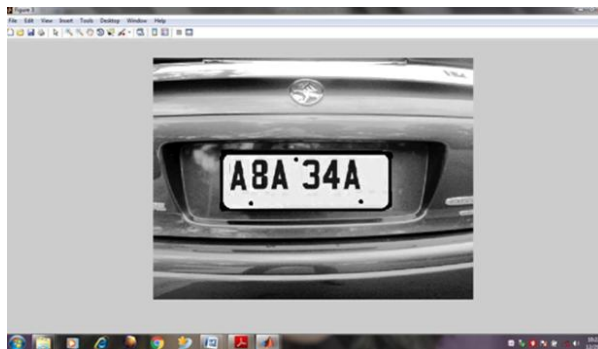
Fig 4: Image after Histogram Equalization
