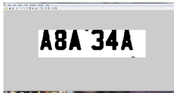
Fig.9: Image after morphology operation imopen
