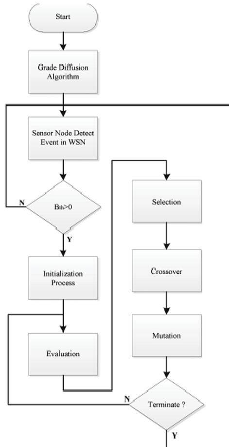
Fig 2. Algorithm Related to Fault Node Recovery
