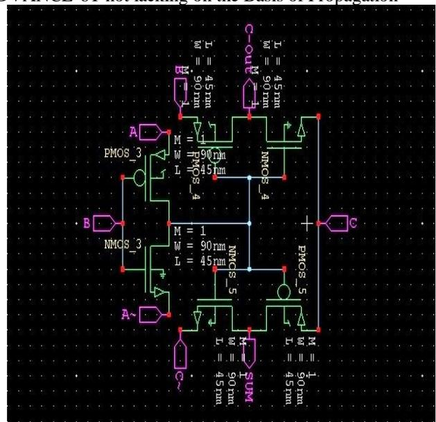
Fig. 7 Schematic Design of Advance 6T Full Adder
