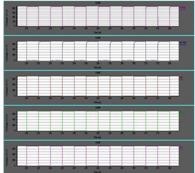
Fig. 9 Simulation Wave form of Advance 6T Full Adder at 45nm
