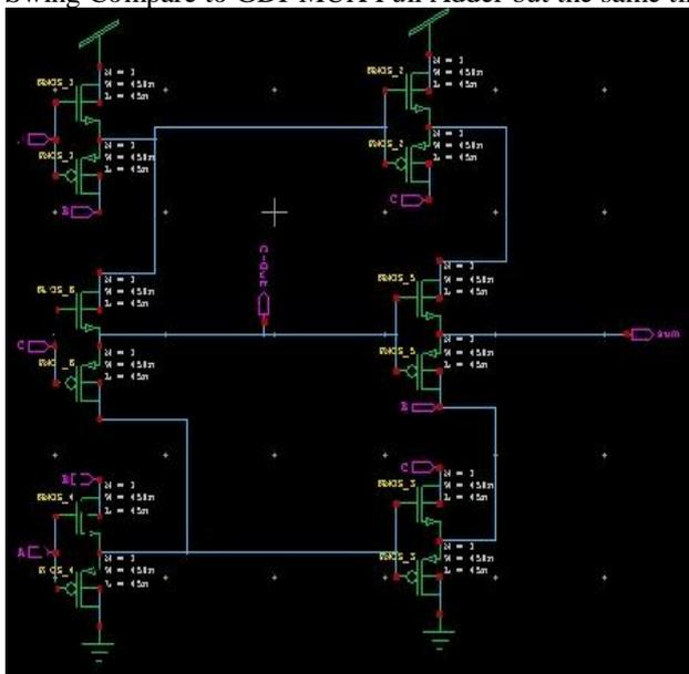
Fig. 4 Schematic Design of GDI-MUX Full Adder
