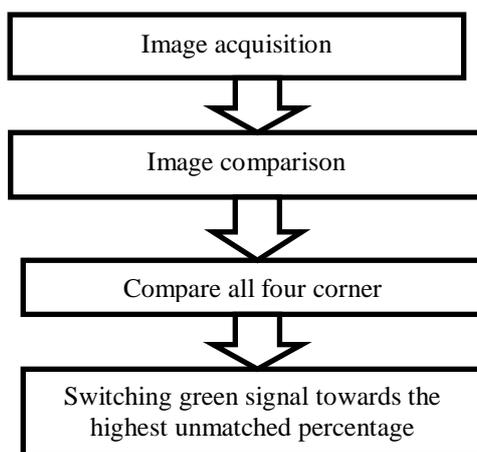
Fig:1- Block diagram-Proposed model (for square)
