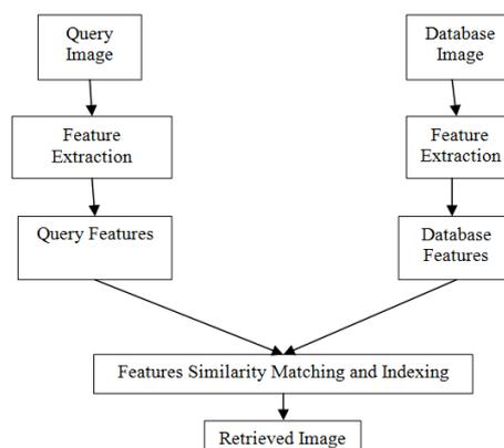
Fig 1 Process flow of Image Retrieval System
