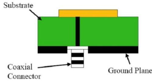
Fig. 4: Coaxial feed Technique
