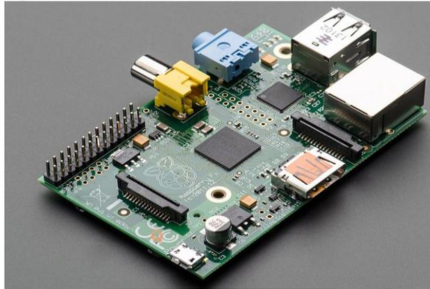
Fig. 1 A RaspberryPi Model B
