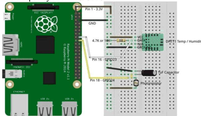
Fig. 5 Connections of the circuit
