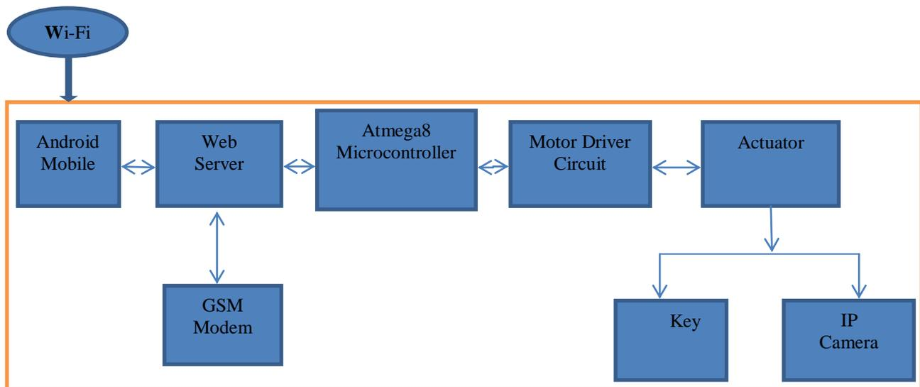
Figure2: Block Diagram of the System
