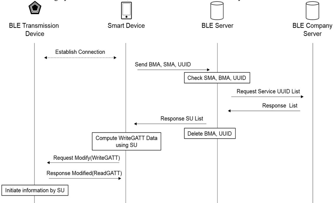
Figure 4 Procedure of deletion BLE transmission device
