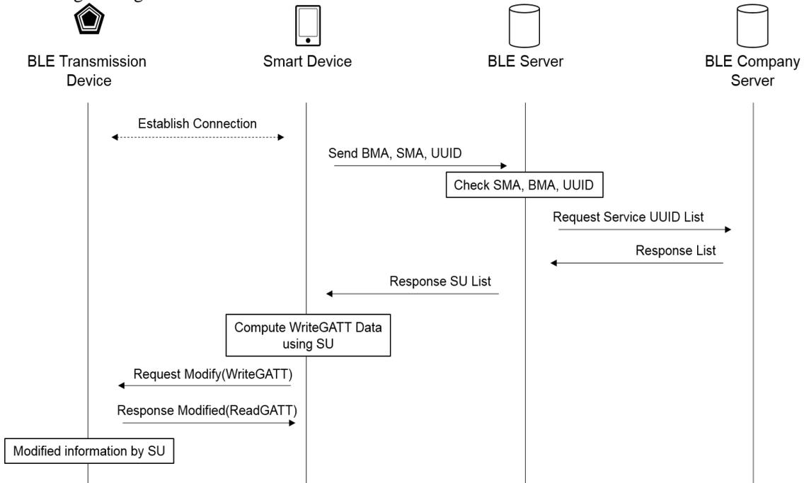
Figure 3 procedure of BLE transmission device modification
