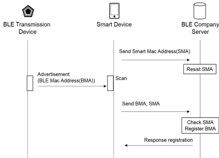
Figure 2 procedure of BLE transmission device, and smart device enrollment
