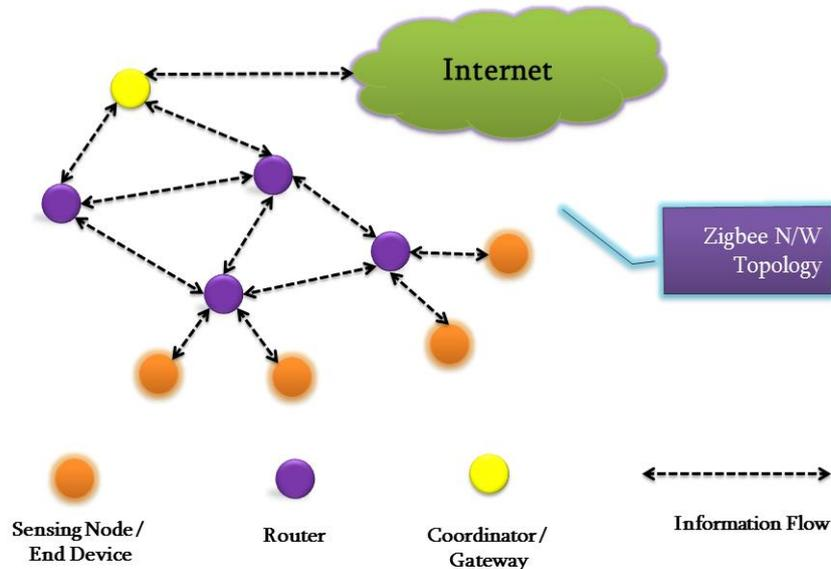
Fig3. Working of Zigbee Devices
