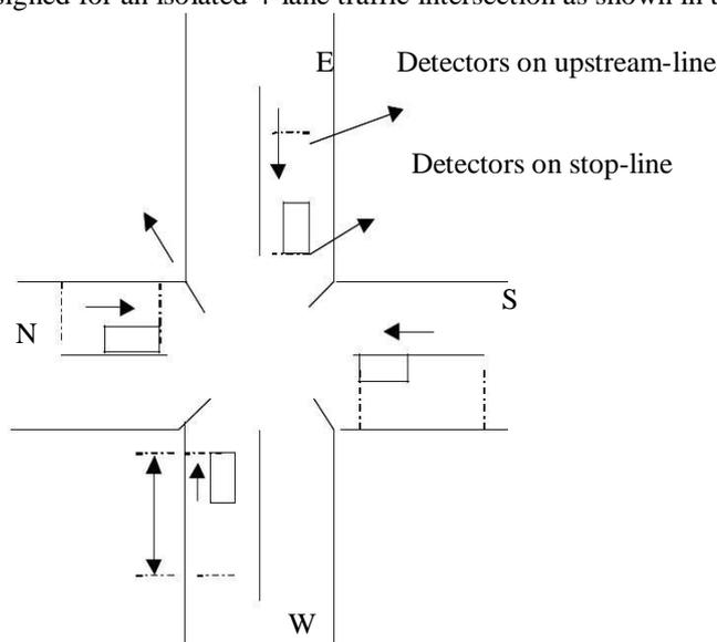
Figure 2: An intersection with detector configuration
