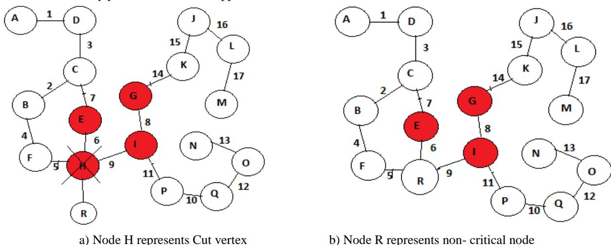
Fig 3: Recovery Procedure when Backup Node is Non-Cut vertex. a) Node H is cut vertex & its backup R is no-cut vertex. b) R simply replaces the failure node H.
