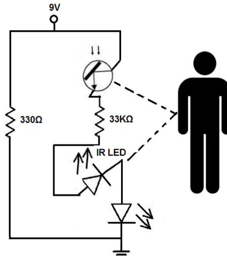
Fig. 2 IR sensor Schematic Diagram
