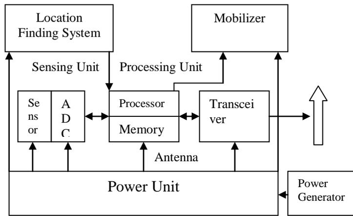
Fig 2: Block diagram sensor networks
