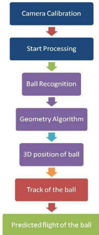
Fig. 1: Hawk-Eye Flow Diagram
