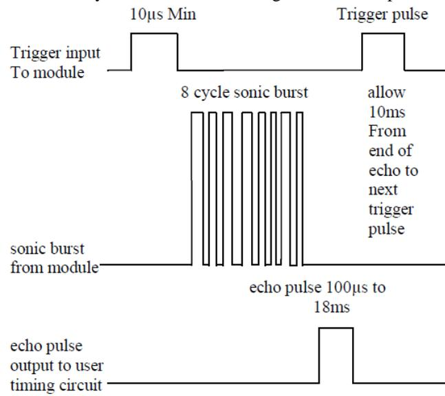
note: echo pulse is approx 36ms if no object is detected
