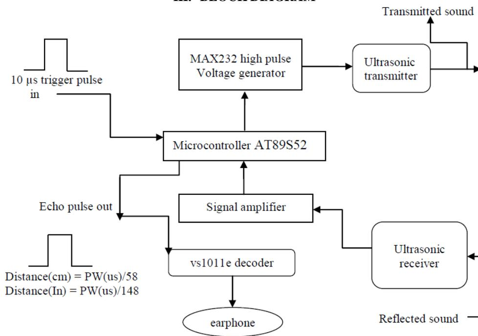
Figure 1: Block diagram of echo based obstacle detector
