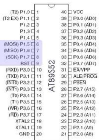
Figure 4: PIN diagram of AT89S52 [16]
