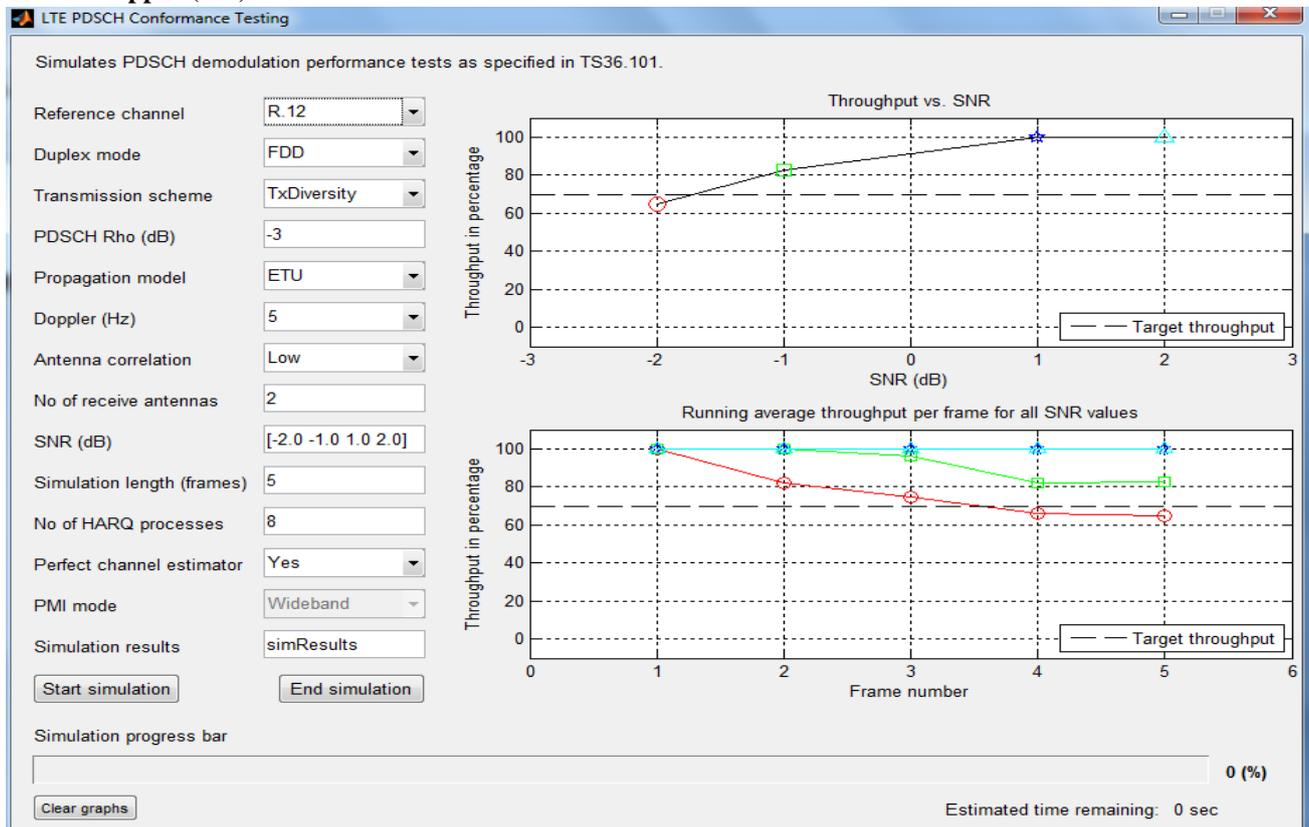
Figure 3: : % throughput for SNR & no. of frames (5 hz doppler)
