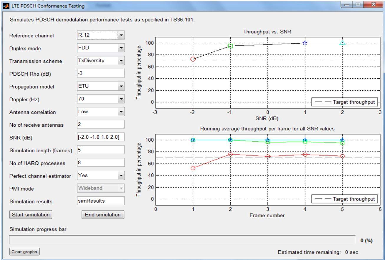
Figure 4: % throughput for SNR & no. of frames (70 hz doppler)
