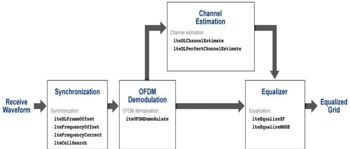
Figure 2: PDSCH downlink receiver function
