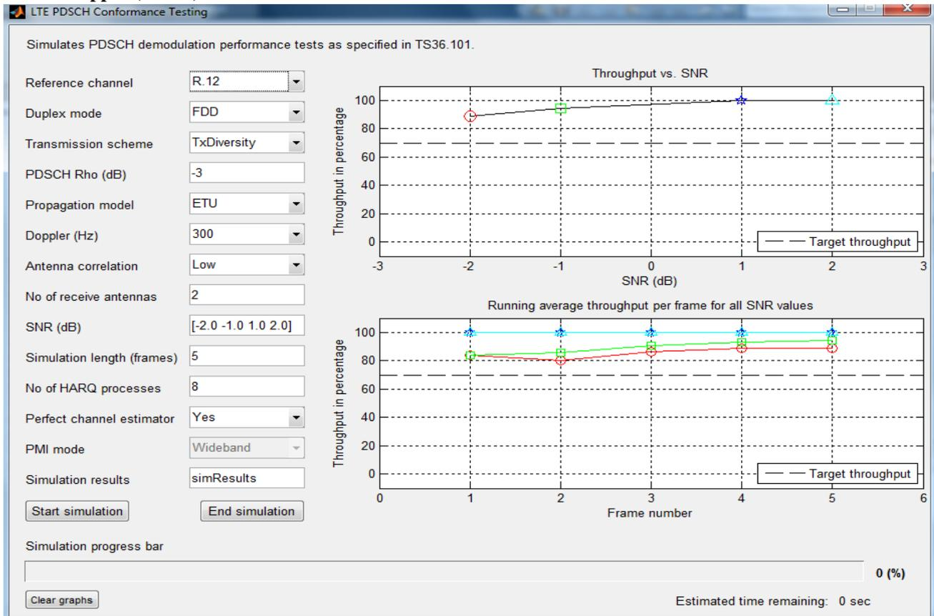
Figure 5: % throughput for SNR & no. of frame (300 hz doppler)
