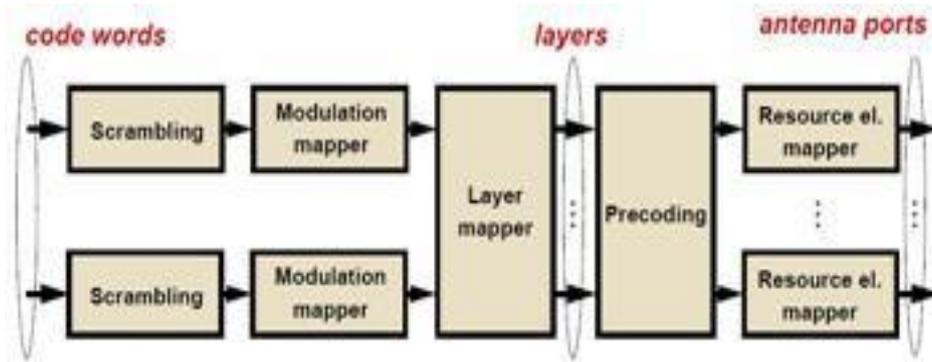
Figure 1: LTE PDSCH downlink channel
