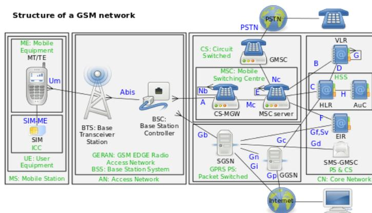
Fig.1: Structure of GSM network
