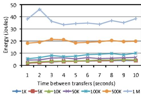
(b) GSM: Varying inter-transfer times
