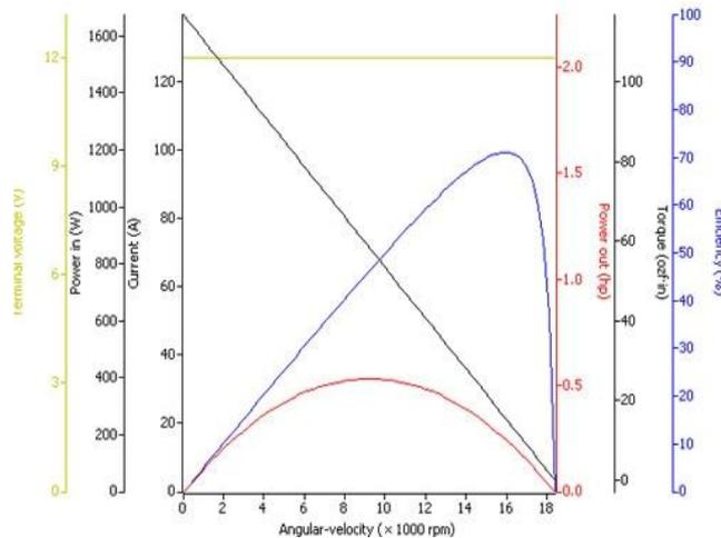
Fig 5:Motor performance graph –voltage ,power, current Torque efficiency.
