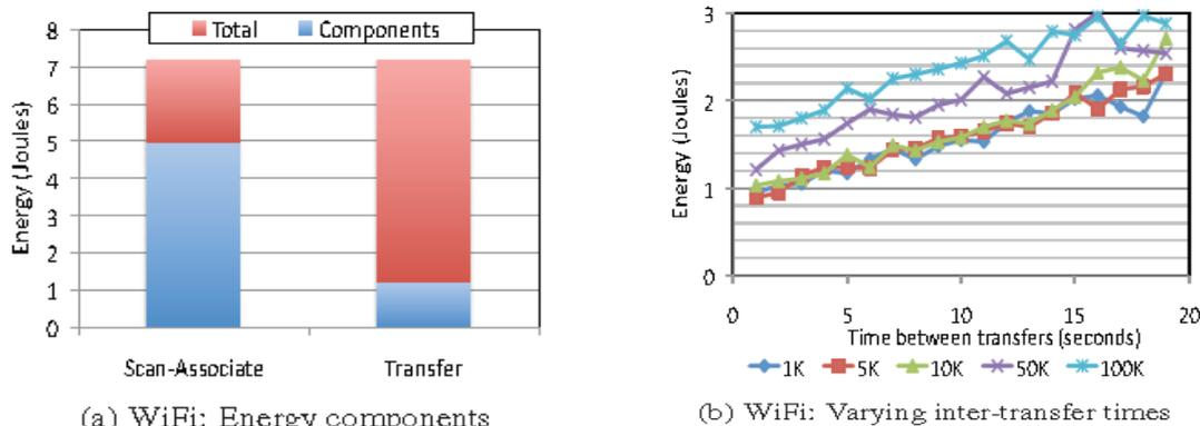
Figure 6: WiFi Measurements: (a) Avg scan/associate and transfer energy consumed to download 50 K data. The lower portion of the stacked columns show the proportion of energy spent on each activity compared to the total energy. (b) Avg energy consumed for downloading data of different sizes against the inter transfer time
