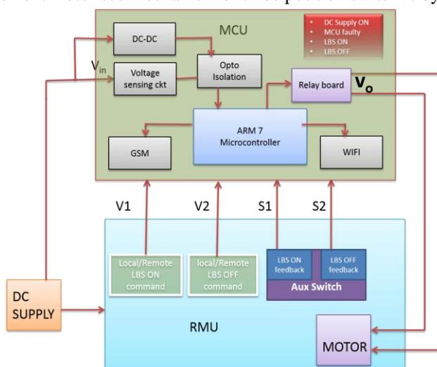
Fig.3: Block diagram of the entire unit
