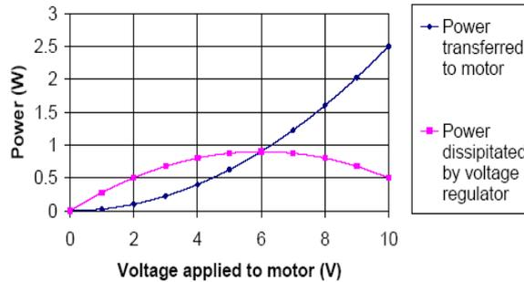
Fig 4 : Power transfer characteristics of voltage contolled motor controller.
