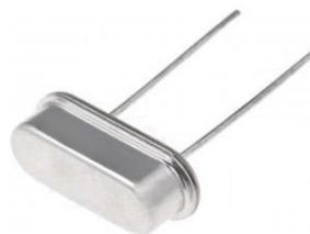
A crystal oscillator is an electronic circuit that uses the mechanical resonance of a vibrating crystal of piezoelectric material to create an electrical signal with a very precise frequency. This frequency is commonly used to keep track of time (as in quartz wristwatches), to provide a stable clock signal for digital integrated circuits, and to stabilize frequencies for radio transmitters/receivers.
