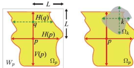
Fig. 5 The left subfigure shows the construction of the shape-adaptive observation window for pixel  $p$ , and the right subfigure shows the weighted aggregation of each  $k \in \Omega_p$
