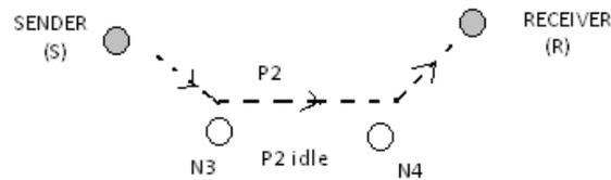
Case iii) If P2 is not idle and P2 is recovered within RTT ,S transmits the frames through P2.
