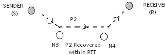
Case iv) If P2 is not idle and P2 is not recovered within RTT ,S transmits the frames through P1.
