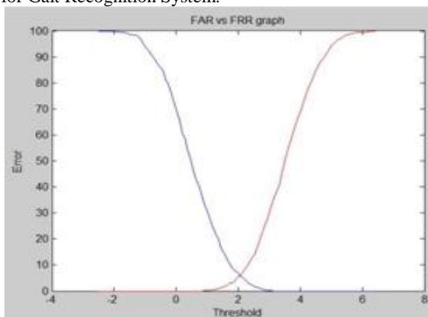
Figure 7: Graphical representation of FAR and FRR for Gait Recognition system under different Threshold Values.
