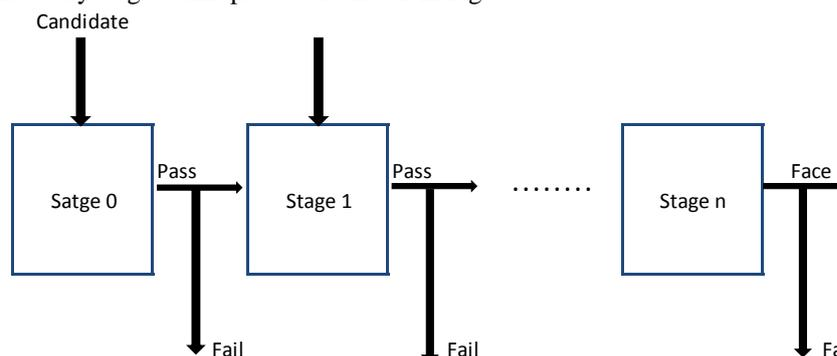
Fig 3. Cascade of stages. Candidate must pass all stages in cascade to be concluded as face.
