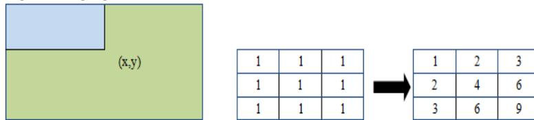
Fig 1. Integral image generation. The shaded region represents sum of pixels up to position (x, y) of image. It shows 3x3 image and its integral image representation.
