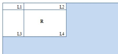
Fig 3. Calculating area of Rectangle R, is done using corner of rectangle :  $L4-L3-L2+L1$ .
