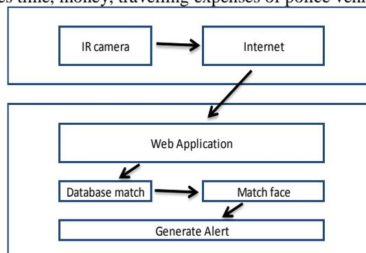
Fig 5. System Architecture for Smart System Recognition.
