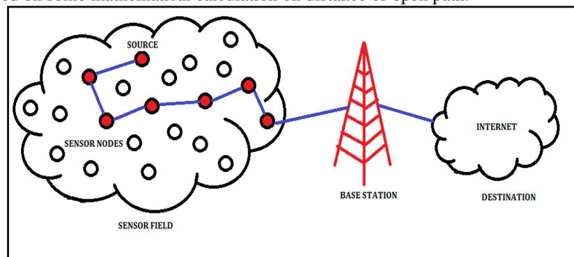
Fig. 1 Routing in Wireless Sensor Network
