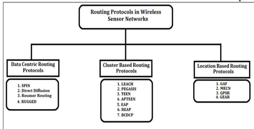
Fig.2 Routing Protocols in Wireless Sensor Network
