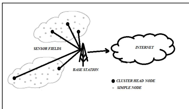
Fig. 5 Cluster Based Routing Techniques
