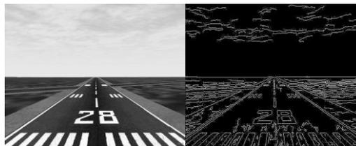
Figure 1: Different edge operator original grayscale Image of the runway and detection by canny edge operator
