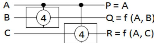
Fig. 5 Symbolic representation of Balanced Quaternary Double Feynman Gate
