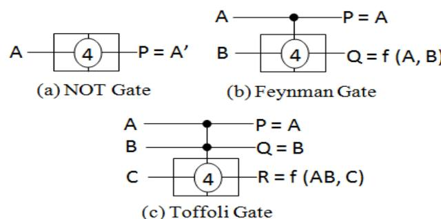
Fig. 3 Balanced Quaternary: (a) NOT Gate, (b) Feynman Gate and (c) Toffoli Gate
