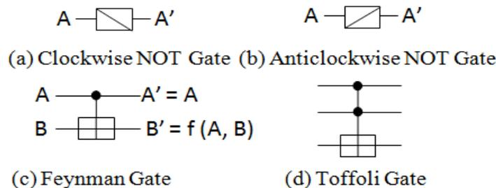
Fig. 2 Balanced Ternary: (a) Clockwise NOT Gate, (b) Anticlockwise NOT Gate, (c) Feynman Gate and (d) Toffoli Gate
