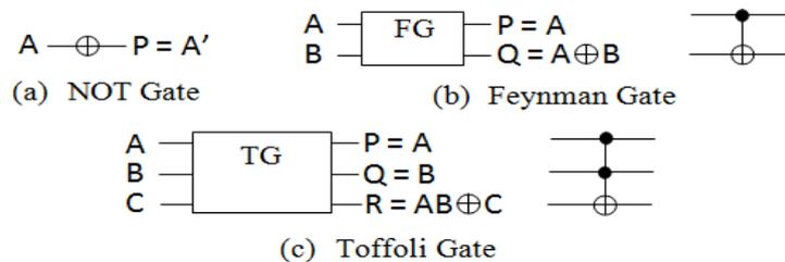
Fig.1 Basic reversible gates: Block diagrams and symbolic forms.
