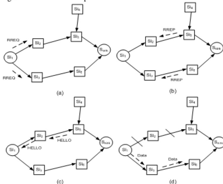
Fig. 2. C-AODV Protocol architecture
