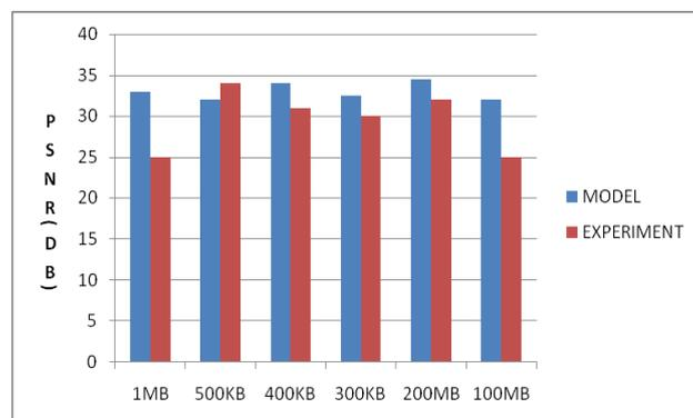
Figure 3 – Estimated versus observed PSNR of decoded video at different bandwidths
