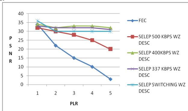
Figure 2 – PSNR of decoded video versus PLR
