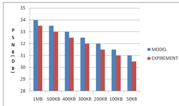
Figure 4 – Estimated versus observed PSNR of decoded video at different bandwidths
