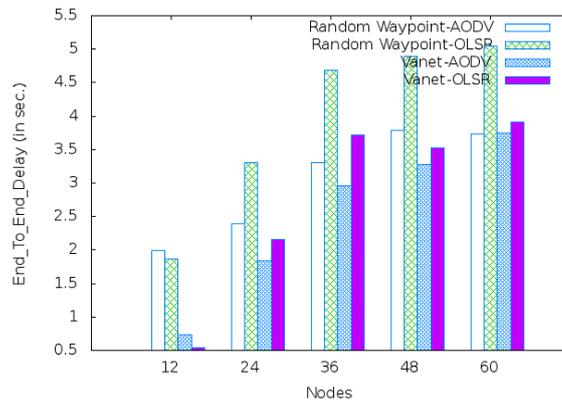
Fig.7. Effect of node density on End to End Delay.
