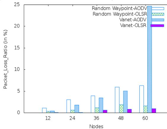
Fig.2. Effect of node density on Packet Loss Ratio.
