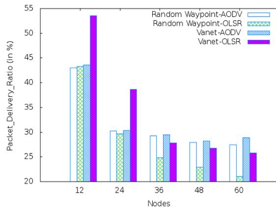
Fig.5. Effect of node density on Packet Delivery Ratio.
