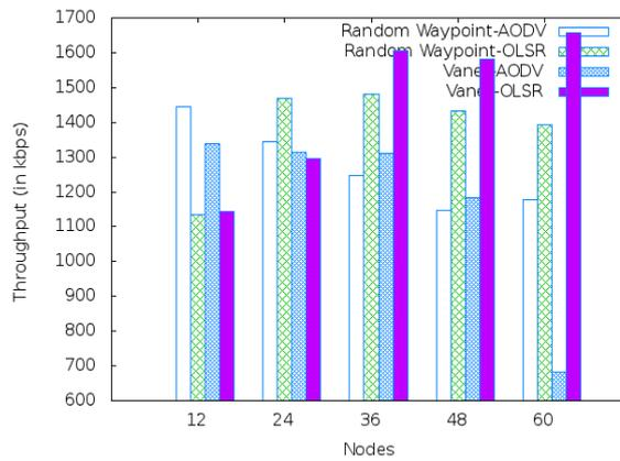
Fig.4. Effect of node density on Throughput.
