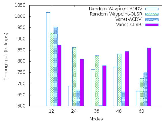
Fig.8. Effect of node density on Throughput.
