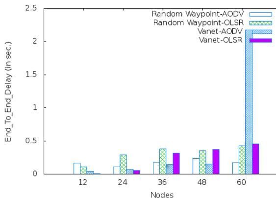
Fig.3. Effect of node density on End to End Delay.
