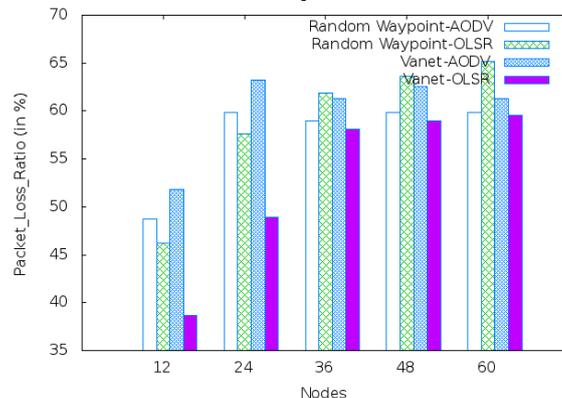
Fig.6. Effect of node density on Packet Loss Ratio.
