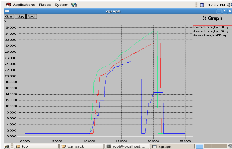
Figure 3: X-Graph representing throughput for TCP-SACK Simulation with 50 nodes in AODV, DSDV & DSR.
