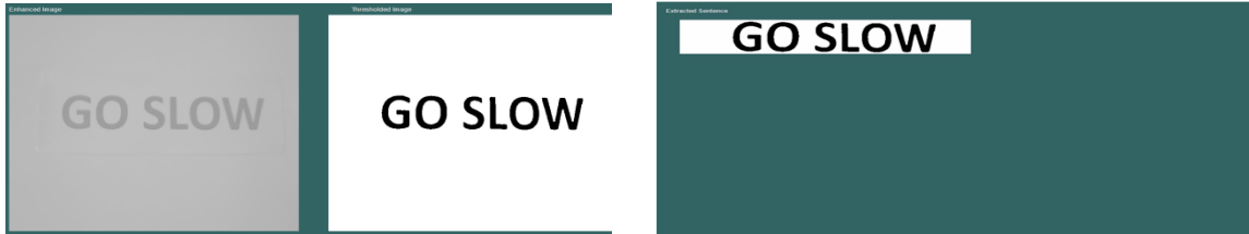
Fig 11: Binarisation is applied to enhanced image. Fig 12: Text extraction from sentence image
