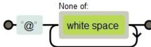
Fig 6: Finite automata representation of Regular Expression for @ Removal
