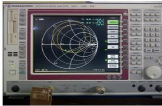
Fig. 6. Antenna connected to the ROHDE network analyzer showing smith chart.
