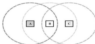
Figure 1: A Mobile Ad hoc network of three nodes, where nodes A and C must discover the route through B in order to communicate.
