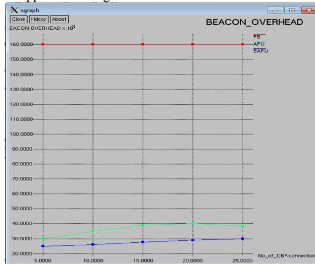
Fig 8 Beacon Overhead Vs Number of CBR Connections
