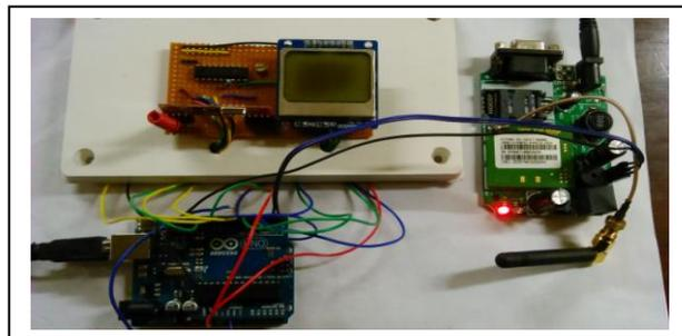
Figure 3(a): Completed Circuit (Dashboard)
