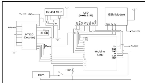
Figure 2(a): Circuit Diagram (Dashboard)
