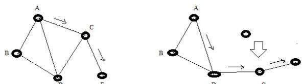
Figure2. Change in Topology due to Movement of node C
