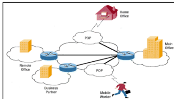
Figure 2: A typical VPN might have a main LAN at corporate office of a company, other LANs are at remote offices and individual users are connecting from out in the field. [8]
