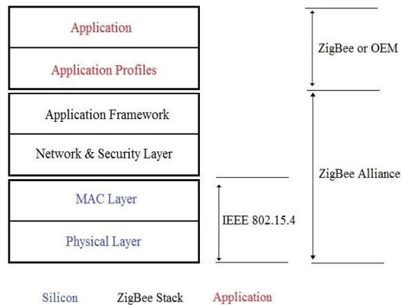
Figure 1 ZigBee Architecture
