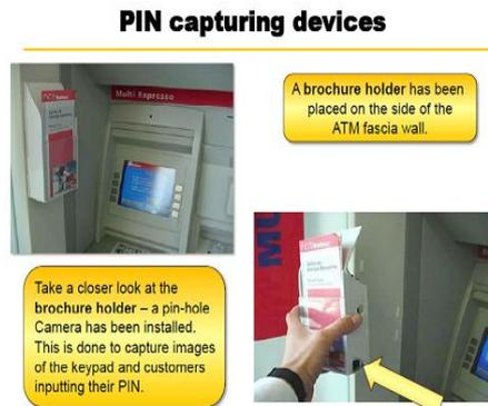
Fig. 5. PIN capturing devices.
