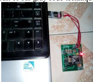
Fig 2: Connection of CC2500 and server
