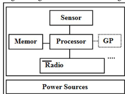
Fig 1. Block diagram for Sensor node
