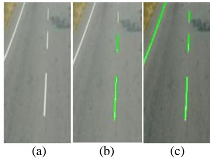
Fig-1 (a) Input image (b) Result of existing approach without using CLAHE technique (c) Result using CLAHE method
