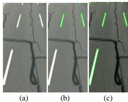
Fig-2 (a) Input image (b) Result of existing approach without using CLAHE technique (c) Result using CLAHE method
