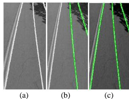
Fig-3 a) Input Image (b) Result of existing approach without using CLAHE technique (c) Result using CLAHE method
