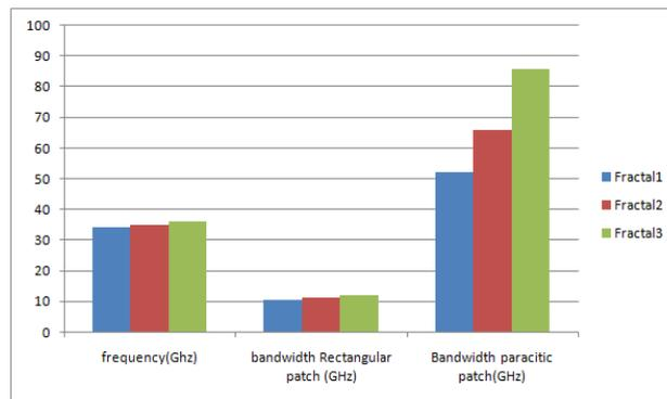
Figure: 3 Bandwidth of Rectangular Fractal and U Slot Fractal Antenna
