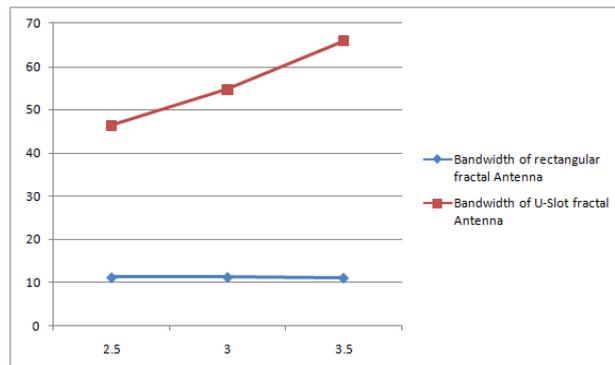
Figure: 5 Bandwidth of Rectangular Fractal Antenna with change of permittivity of stack
