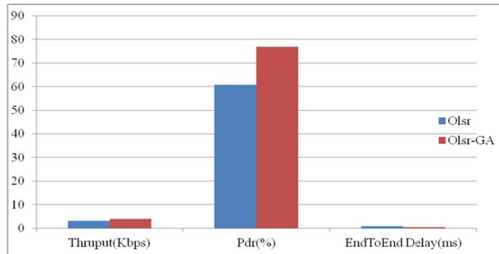
Figure 7. Comparison of Throughput, Pdr, End to End Delay between OLSR and OLSR-GA.
