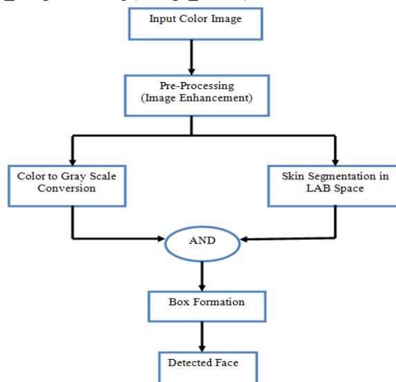
Fig 3. Face detection algorithm
