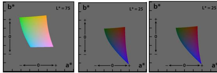
Fig 2. (L\*, A\*, B\*) Color Space (CIELAB), Showing Only Colors That Fit Within the SRGB
