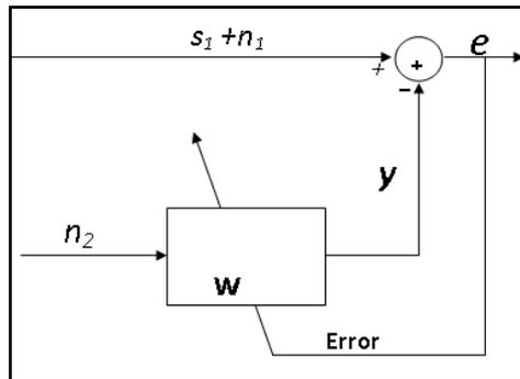
Fig.1. Magnetization Adaptive Filter Structure
