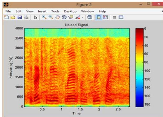
Fig 3. Spectrogram of noisy signal
