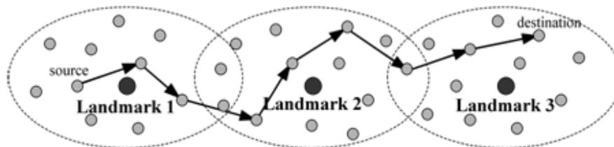
LANMAR Routing in an Ad Hoc Network without Backbones
