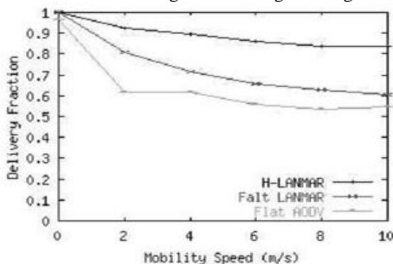
Fig. 2: Comparison of delivery fraction vs. mobility
