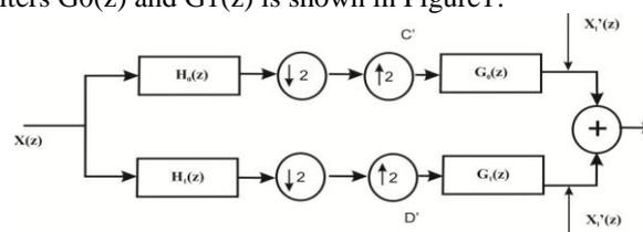
Figure 1 DWT Filter Bank
