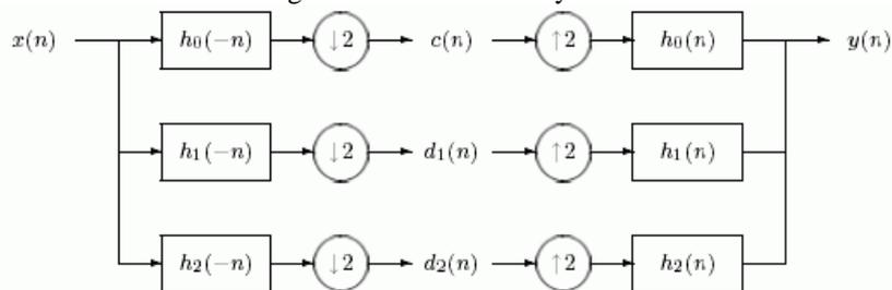
Figure 3: A 3-Channel Perfect Reconstruction Filter Ban
