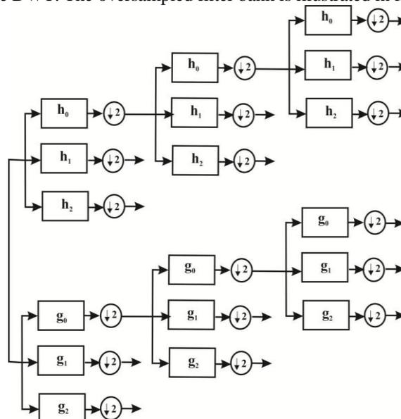
Figure 5 Iterated Filter Bank for Double Density Complex DWT
