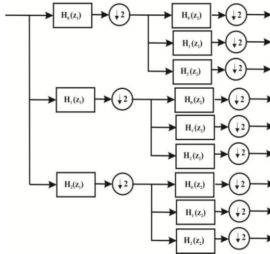
Figure 4 An over sampled Filter Bank
