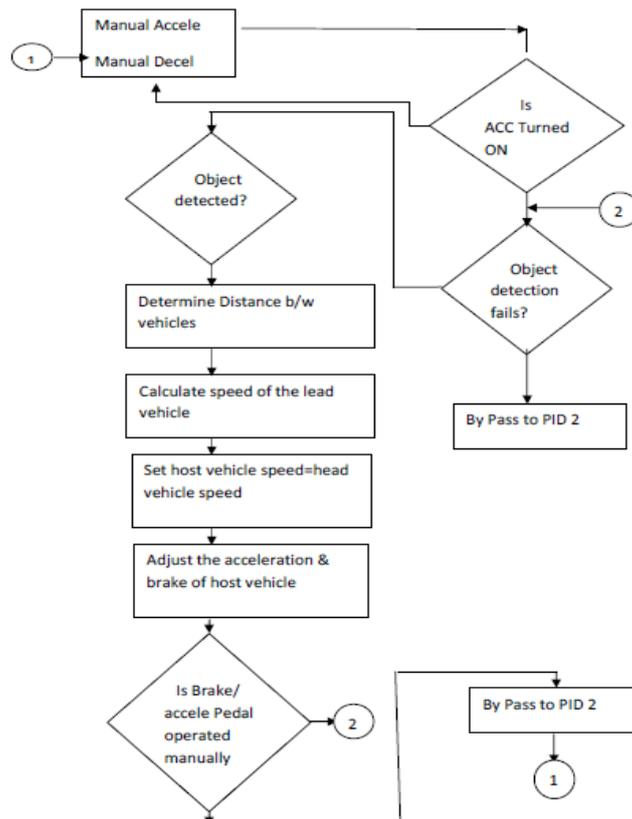
Figure 2: Flow Chart of New Adaptive Cruise Control
