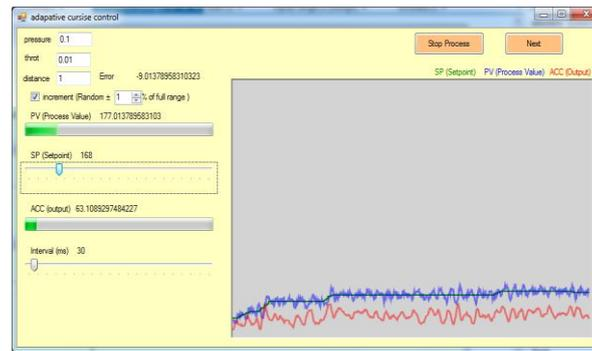
Figure 7: Simulation of Adaptive Cruise Control System using Window Form
