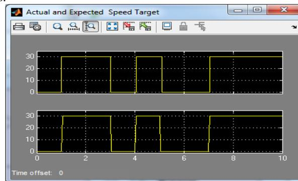
Figure 8: Actual and Expected speed of the Adaptive Cruise Control System
