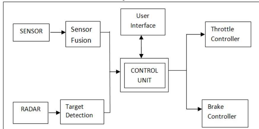
Figure 1: Architecture of Adaptive Cruise Control System
