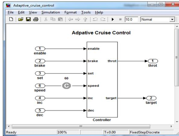
Figure 4: Adaptive Cruise Control (ACC) circuit
